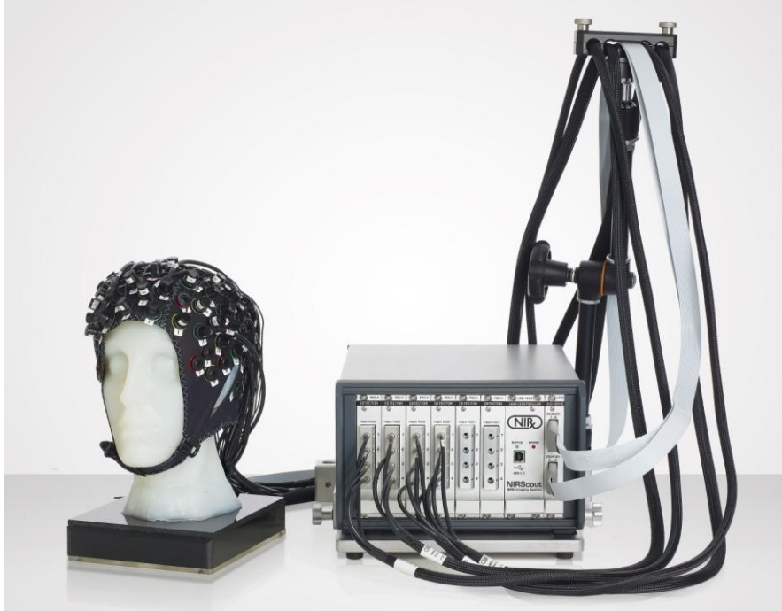
Fig. 4: Complete measurement setup (control PC not shown). (1) NIRScout-1624 imaging system, configured for a 16-source-by-16-detector measurement. (2) Source optode cables; (3) Fiber optic detector cables; (4) articulating arm with (5) base plate and (6) cable clamp for strain relief; (7) Head phantom.
