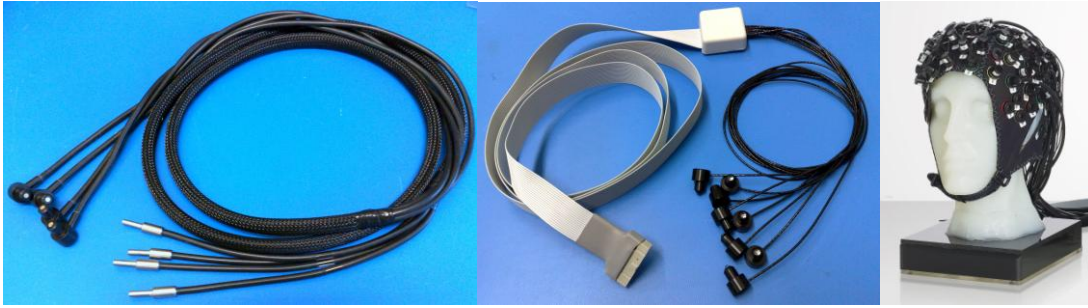
Fig. 3: Sensors used with the NIRScout system. (a) Detection fiber optical cables, bundle of four. The black plastic tips are placed on tissue, the metal end ferrules are inserted into the detection card. (b) Bundle of eight dual-wavelength LED emitters. Black plastic ends with LED lens are placed on the skin, and the ribbon cable connects to the LED driver card. (3) Example of optode placement on a Phantom head.
