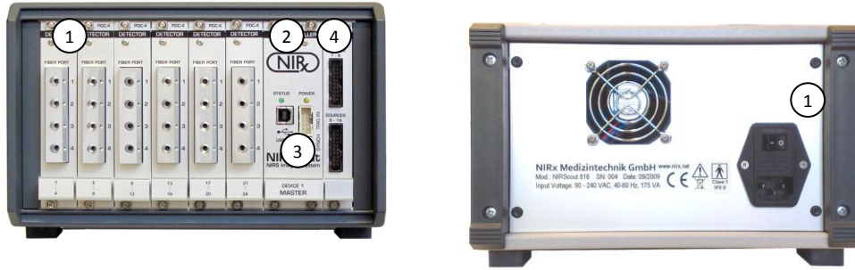
Fig. 2: (a) Front view of the NIRScout 816 imaging system. (1) Quad-channel detection cards QDC-10; (2) USB controller card USB-1618 with Trigger input (3); (4) Led driver card LED-16. (b) Rear View showing AC power inlet and power main On/Off switch (1).
